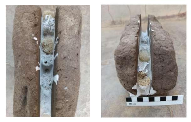
Grouting tests with Luffa pieces, filled between two mud bricks found in the desert
